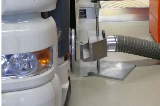
Exhaust gas extraction unit
